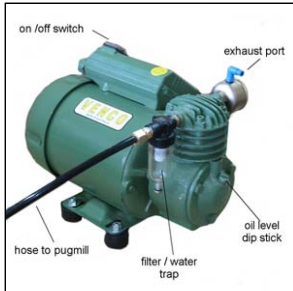
Figure 3: Vacuum hose and filter location on the vacuum pump
